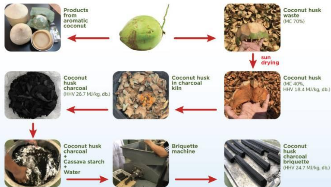
Properties of coconut husk charcoal briquette vs. raw coconut husk
