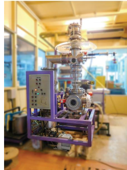
Fig. 1. Low-energy ion bombardment for mutation induction in SYP rice seeds: (a) the vertical compact ion implanter, (b) inserting dehulled SYP rice grains into a copper samole holder, and (c) embryo, the target area, at the surface of a dehulled SYP rice grain.
